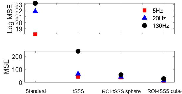
**FIGURE 3** The mean squared error (MSE) of the simulated dipole topography, computed between different DBS conditions and the no stimulation condition is plotted for all four pre-processing approaches in the phantom recording. The lowest MSE across all stimulation conditions is achieved by the ROI-tSSS sphere and the ROI-tSSS cube approaches. The ROI-tSSS approaches offer the greatest benefit at clinically deployed DBS frequencies of 130 Hz.
